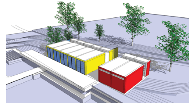
4. Coloured panels and roof SIPS
